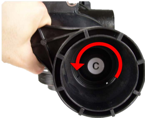
Use the closed end of service wrench to loosen injector cap
