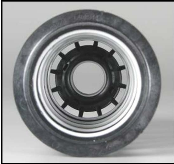
Pull out the spacer stack assembly
