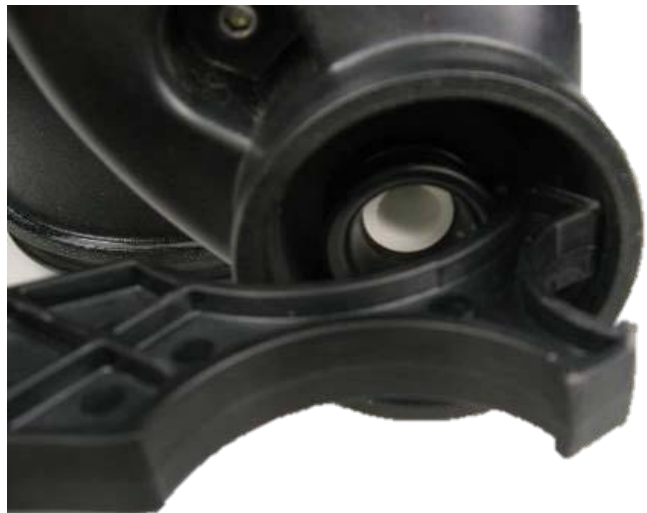
Gently pry the injector with open end of service wrench
