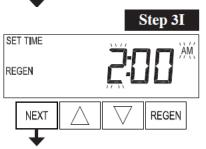
**Step 3I** – Next Regeneration Time (hour): Set the hour of day for regeneration using ▲ or ▼. The default time is 2:00.
