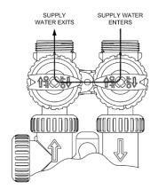
To shut off supply to the Unit the bypass valve handle must be in direction given above.
