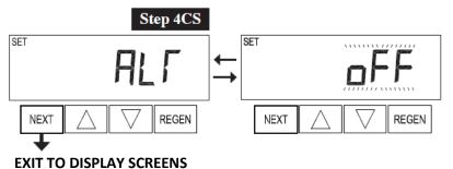
Step 4CS – Select "OFF" when none of features are used using ▲ or ▼ buttons. Press NEXT to exit Configuration Settings. Press REGEN to return to previous step.
