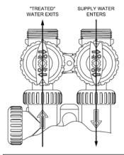
The inlet handle arrow must be in the direction of unit and outlet handle must direct away from the unit as given above.
