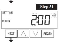
Step 3I – Next Regeneration Time (hour): Set the hour of day for regeneration using ▲ or ▼. The default time is 2:00.
