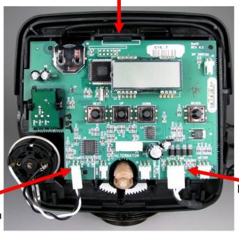
Disconnect Motor Wire 2<sup>nd</sup> Disconnect Power 1st
