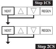
Step 1CS – Press NEXT and ▼ simultaneously for 5 seconds and release. Press NEXT and ▼ simultaneously for 5 seconds and release. If the screen in Step 2CS does not appear, the lock on the valve is activated. To unlock, press ▼, NEXT, ▲ and REGEN in sequence, then press NEXT and ▼ simultaneously for 5 seconds and release. Press NEXT and ▼ simultaneously for 5 seconds and release.
