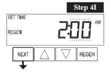
**Step 4I** – Next Regeneration Time (minutes): Set the minutes of day for regeneration using ▲ or ▼. This display will not be shown if "on 0" is selected in Set Regeneration Time Option in OEM Filter System Setup or OEM Filter System Setup.
