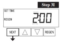
**Step 3I** – Next Regeneration Time (hour): Set the hour of day for regeneration using  $\triangle$  or  $\nabla$ . The default time is 2:00.
