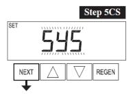
**Step 5CS** – Select feature "SYS" using ▲ or ▼ buttons for filters.
