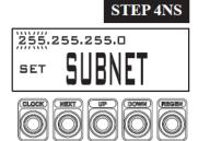
**STEP 4NS:** - Subnet Masking – Set the proper Subnet Mask. Each Subnet Mask has four sections separated by decimal points. The System Controller will only be able to communicate with other devices within the same subnet. Pressing CLOCK will select the first section of the address to be changed by pressing UP or DOWN buttons to adjust each section. Pressing NEXT will advance to the next section and to the Step 5NS.
