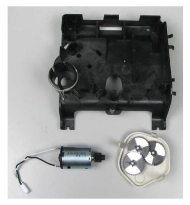
Motor can be removed by pressing the locking spring to the right and then pull the motor out. Gearbox can be removed by pushing the beige colored locking tabs inwards.
