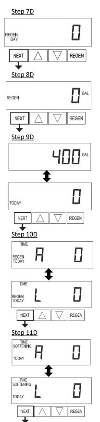
**Step 7D**: - This display shows the days since the last regeneration occurred. Press NEXT to go to Step 8D. Press REGEN to return to previous step.
