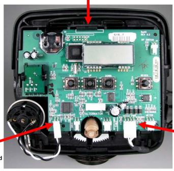
Disconnect Motor Wire 2<sup>nd</sup> Disconnect Power 1st
