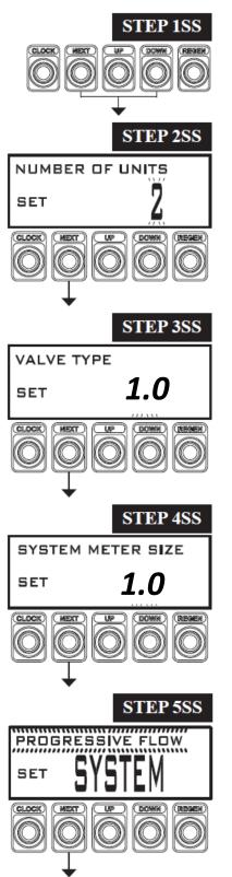
**STEP 1SS:** - Press NEXT and DOWN simultaneously for three seconds and release.
