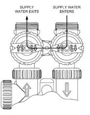
**Normal Position:** - The inlet and outlet valve must be fully open and bypass valve must be fully closed.
