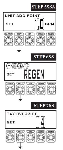
**Step 5SSA:** - Adjust the unit add point in GPM as specified on the specifications of the system model. Press NEXT to go to Step 6SS.
