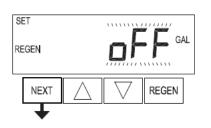
**Step 5F** – Set the regeneration trigger using  $\blacktriangle$  or  $\triangledown$  to adjust the number of gallons as per specifications of filter model.
