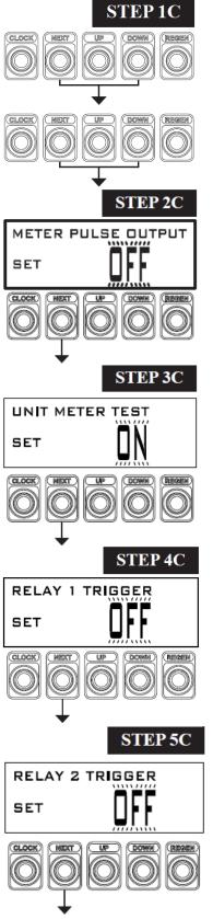
**STEP 1C:** - Press NEXT and DOWN simultaneously for approximately three seconds, then release. Press NEXT and DOWN again simultaneously for 3 seconds and release.
