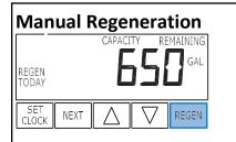
**Immediate Regeneration:** - Press and hold "REGEN" button for more than 3 seconds. Press "REGEN" button to advance the unit to next cycle in regeneration.
