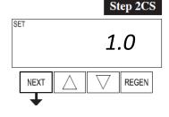
**Step 2CS** – Use  $\blacktriangle$  or  $\triangledown$  to select **1.0** for 1.0" valve. Press NEXT to go to Step 4CS. Press REGEN to exit Configuration Settings.
