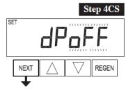
**Step 4CS** – Select dP OFF - outside regeneration signal feature not used, by using  $\blacktriangle$  or  $\triangledown$  buttons.
