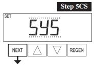
**Step 5CS** – Select feature "SYS" using ▲ or ▼ buttons for filters.
