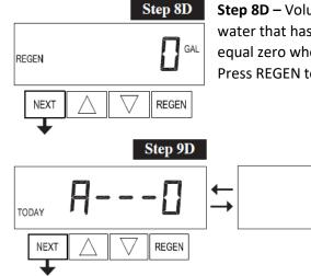
**Step 8D** – Volume, since last regeneration: This display shows the volume of water that has been filtered since the last regeneration. This display will equal zero when a water meter is not installed. Press NEXT to go to Step 9D. Press REGEN to return to previous step.
