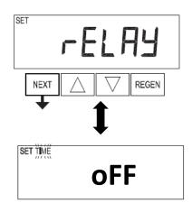
**Step 6S** – Select relay operation "oFF" using  $\blacktriangle$  or  $\blacktriangledown$  buttons. Press NEXT to exit filter system setup.
