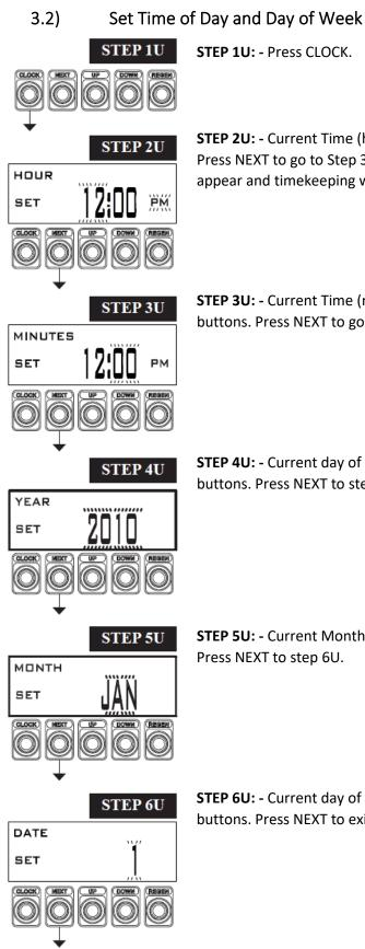
STEP 2U: - Current Time (hour): Set the hour using UP or DOWN buttons. Press NEXT to go to Step 3U. With metric units set, AM/PM indication will not appear and timekeeping will be shown in the 24-hour format.
