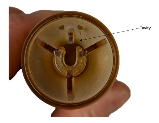
The main piston is attached with snap off connection.
