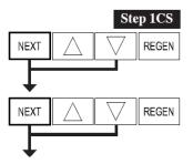
activated. To unlock, press ♥, NEXT, ▲ and REGEN in sequence, then press NEXT and ♥ simultaneously for 5 seconds and release. Press NEXT and ♥ simultaneously for 5 seconds and release.
