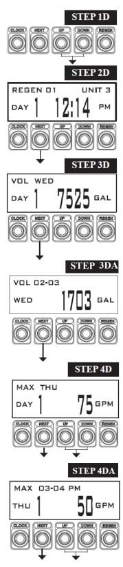
**STEP 1D: -** Press UP and DOWN buttons simultaneously for three seconds and release.
