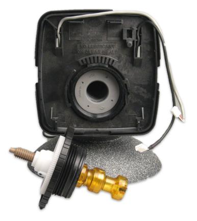
Pull out the drive cap with main piston.
