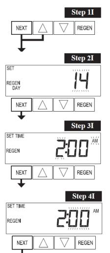
**Step 1I** - To enter Installer Display press NEXT and ▲ simultaneously for about 5 seconds and release.
