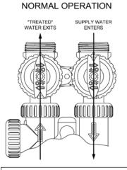
The inlet handle arrow must be in the direction of unit and outlet handle must direct away from the unit as given above.
