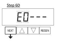
**Step 6D**: - This display shows a history of the last 10 errors generated by the control during operation. Press  $\blacktriangle$  or  $\blacktriangledown$  to view each recorded error.
