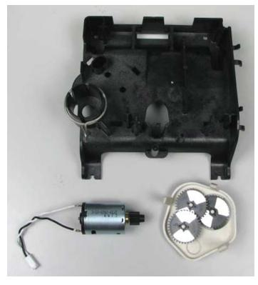
Motor can be removed by pressing the locking spring to the right and then pull the motor out. Gearbox can be removed by pushing the beige colored locking tabs inwards.
