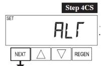
**Step 4CS** – Select "ALT A" or "ALT B" when none of features are used using  $\blacktriangle$  or  $\blacktriangledown$  buttons. Press NEXT to exit Configuration Settings. Press REGEN to return to previous step.
