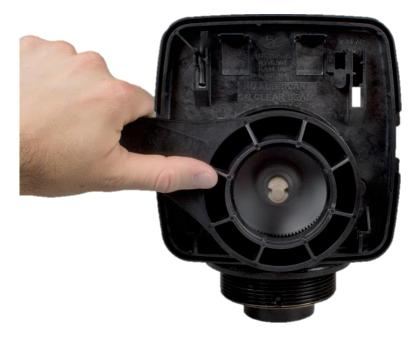
Turn the drive cap counter clockwise with the closed end of service wrench.
