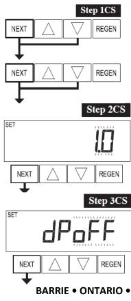
Step 1CS – Press NEXT and ▼ simultaneously for 5 seconds and release. Press NEXT and ▼ simultaneously for 5 seconds and release. If the screen in Step 2CS does not appear, the lock on the valve is activated. To unlock, press ▼, NEXT, ▲ and REGEN in sequence, then press NEXT and ▼ simultaneously for 5 seconds and release. Press NEXT and ▼ simultaneously for 5 seconds and release.
