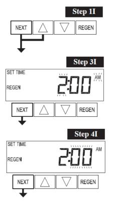
**Step 1I** - To enter Installer Display press NEXT and ▲ simultaneously for about 5 seconds and release.
