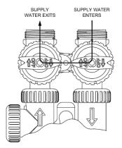
To shut off supply to the Unit the bypass valve handle must be in direction given above.
