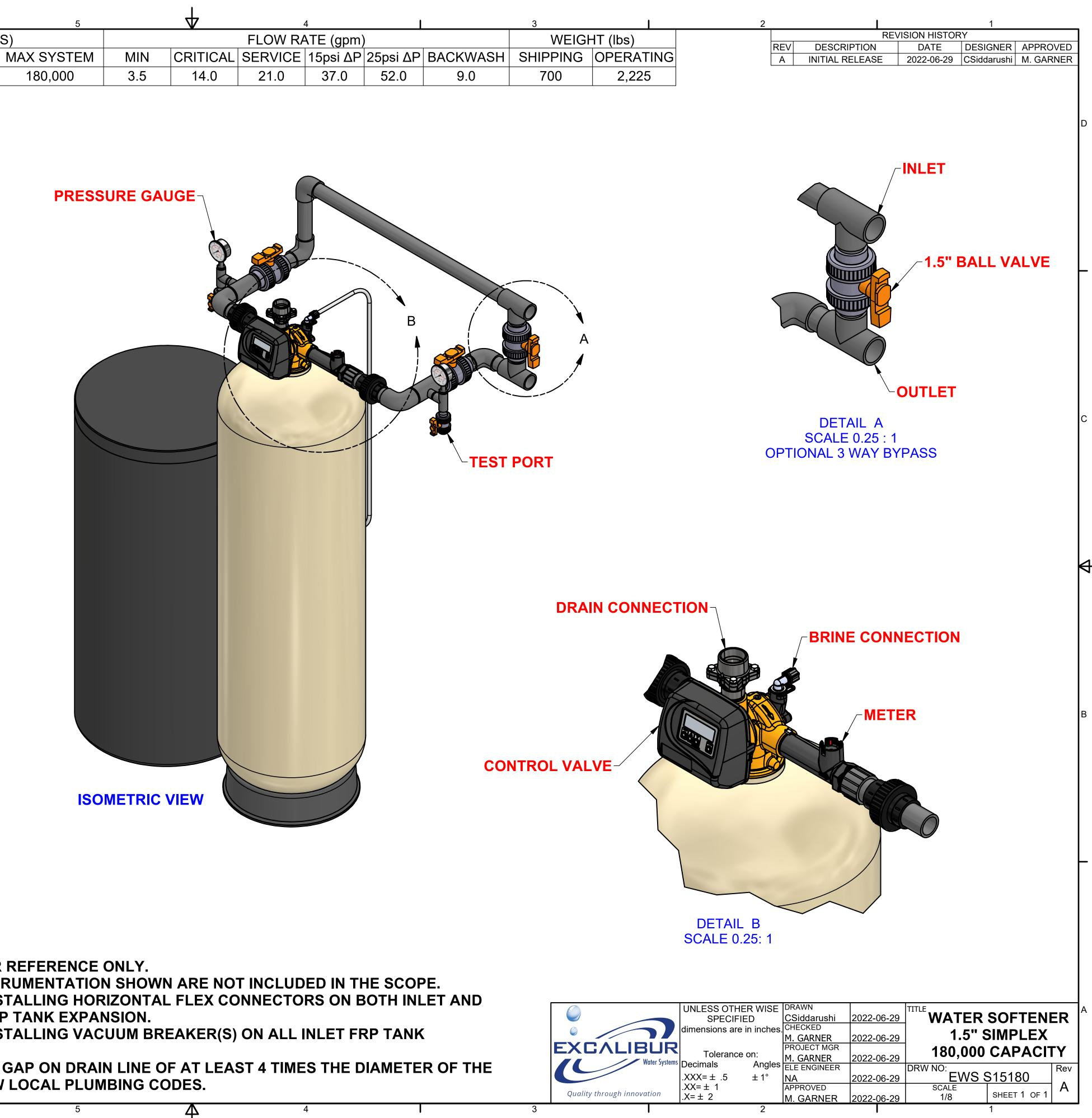
DRAWING IS FOR REFERENCE ONLY. PIPING AND INSTRUMENTATION SHOWN ARE NOT INCLUDED IN THE SCOPE. **RECOMMEND INSTALLING HORIZONTAL FLEX CONNECTORS ON BOTH INLET AND** OUTLET FOR FRP TANK EXPANSION. 4. RECOMMEND INSTALLING VACUUM BREAKER(S) ON ALL INLET FRP TANK 5. PROVIDE AN AIR GAP ON DRAIN LINE OF AT LEAST 4 TIMES THE DIAMETER OF THE PIPE OR FOLLOW LOCAL PLUMBING CODES.
