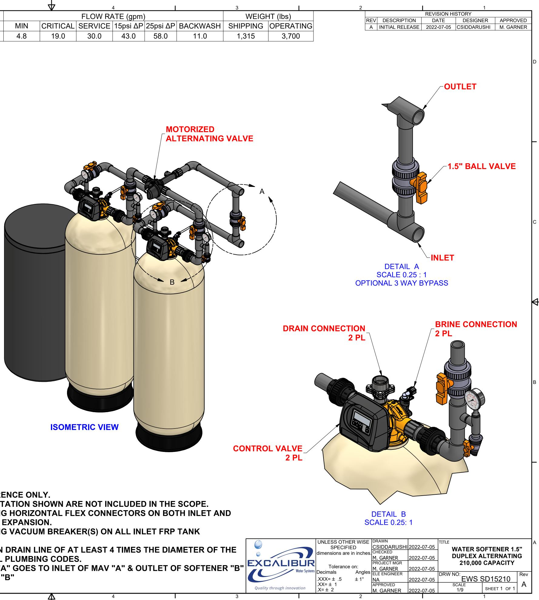
DRAWING IS FOR REFERENCE ONLY. PIPING AND INSTRUMENTATION SHOWN ARE NOT INCLUDED IN THE SCOPE. **RECOMMEND INSTALLING HORIZONTAL FLEX CONNECTORS ON BOTH INLET AND OUTLET FOR FRP TANK EXPANSION.** 4. RECOMMEND INSTALLING VACUUM BREAKER(S) ON ALL INLET FRP TANK CONNECTIONS. 5. PROVIDE AN AIR GAP ON DRAIN LINE OF AT LEAST 4 TIMES THE DIAMETER OF THE PIPE OR FOLLOW LOCAL PLUMBING CODES. 6. OUTLET OF SOFTENER "A" GOES TO INLET OF MAV "A" & OUTLET OF SOFTENER "B" GOES TO INLET OF MAV "B"
