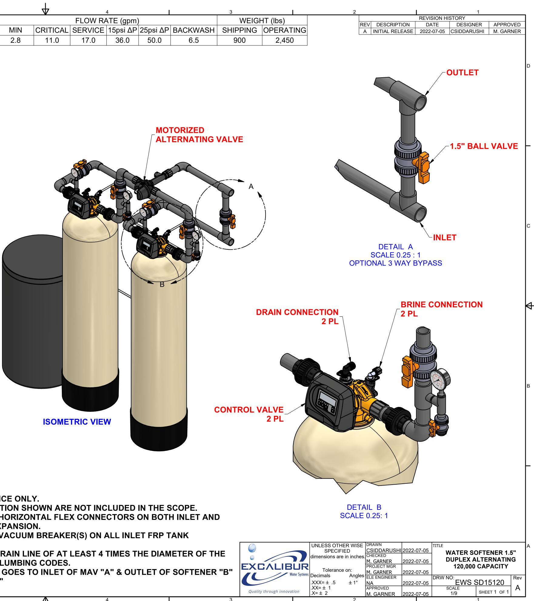
DRAWING IS FOR REFERENCE ONLY. PIPING AND INSTRUMENTATION SHOWN ARE NOT INCLUDED IN THE SCOPE. **RECOMMEND INSTALLING HORIZONTAL FLEX CONNECTORS ON BOTH INLET AND** OUTLET FOR FRP TANK EXPANSION. 4. RECOMMEND INSTALLING VACUUM BREAKER(S) ON ALL INLET FRP TANK **CONNECTIONS.** PROVIDE AN AIR GAP ON DRAIN LINE OF AT LEAST 4 TIMES THE DIAMETER OF THE **PIPE OR FOLLOW LOCAL PLUMBING CODES.** 6. OUTLET OF SOFTENER "A" GOES TO INLET OF MAV "A" & OUTLET OF SOFTENER "B" GOES TO INLET OF MAV "B"
