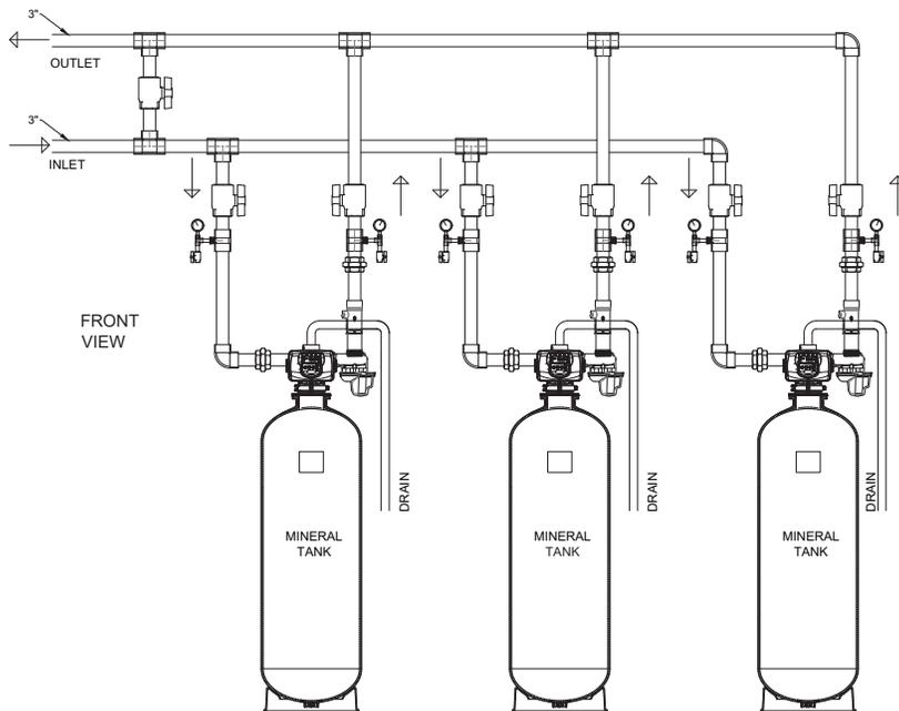
**Triplex & Quadplex Fully Automatic Electronic Demand Industrial Chemical Removal Filters**
